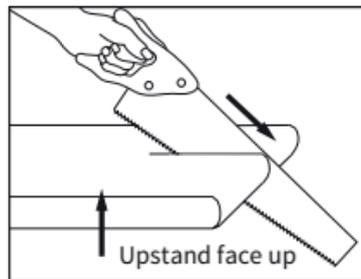
*When using a handsaw the decorative face should be uppermost and again you should start from the decorative profiled front edge keeping the saw at a low angle to ensure the best cut. Ensure that your saw is sharp and well set and has 10/12 teeth per inch.*
