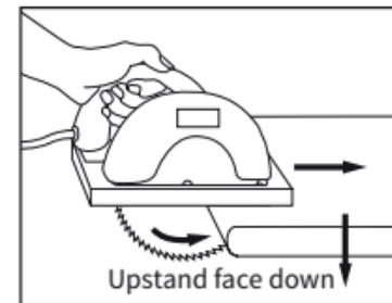
*When using an electric saw you should start from the decorative profiled front edge cutting the upstand face down.*
